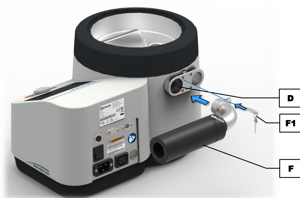
Fig. 2: Mounting the silencer
