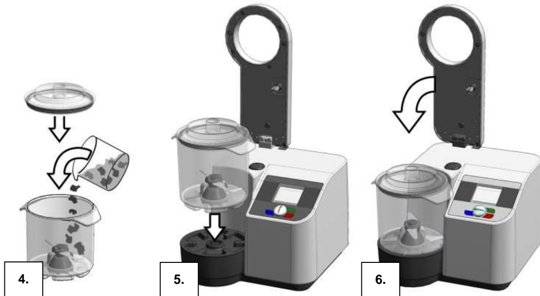
Fig. 12: Inserting the grinding jar and closing the device.
