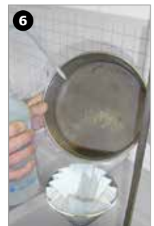
4 Processus de tamisage humide (rinçage + vibration)
