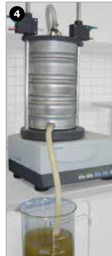
4 Processus de tamisage humide (rinçage + vibration)
