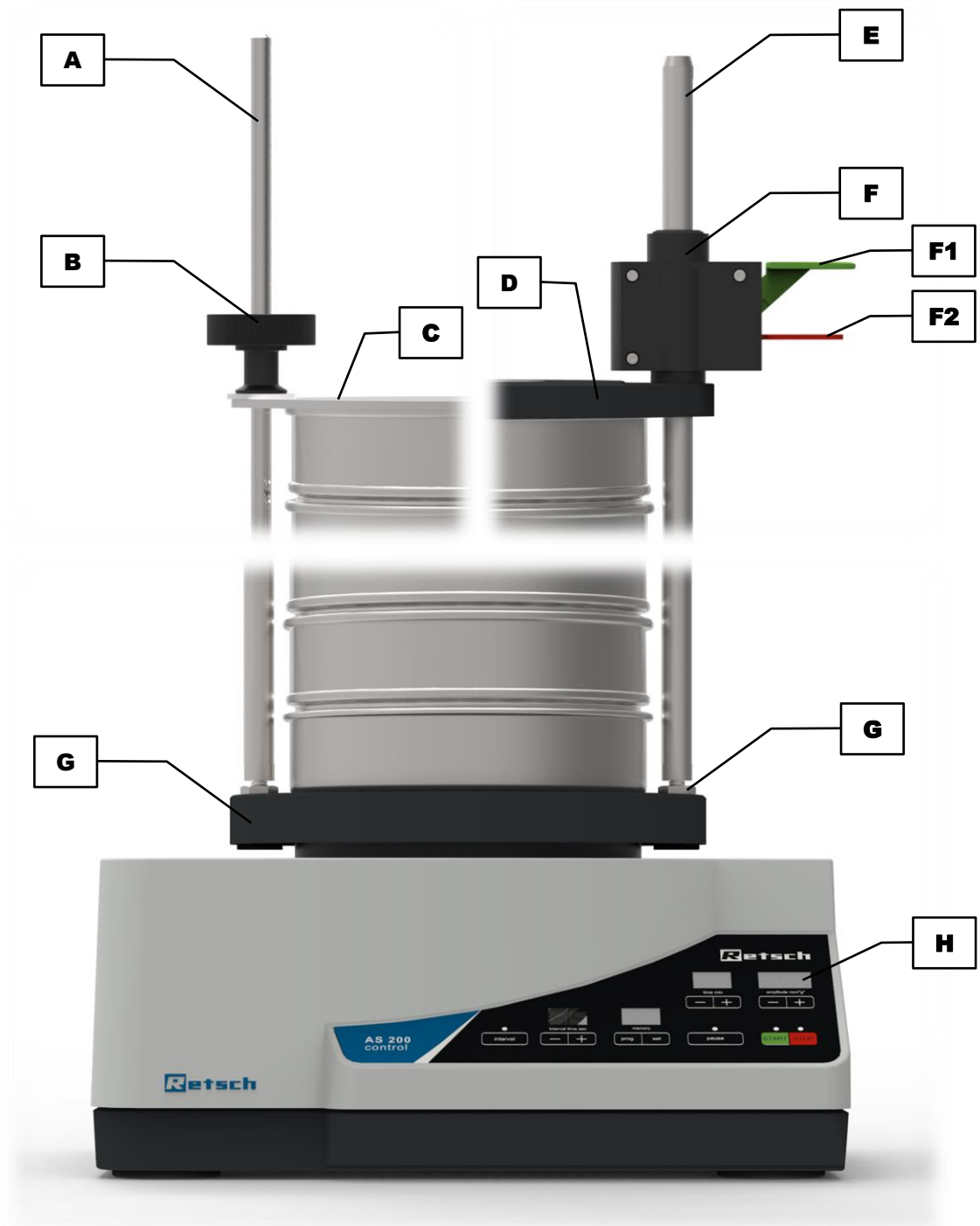
Fig. 7: Front view of the device with different sieve clamping units
