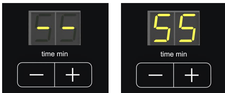
Fig. 11: Time setting for continuous operation (left) or with a process time (right)
