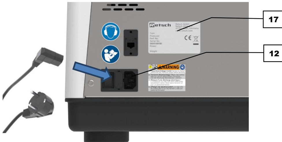
Fig. 9: Facilitating the power connection
