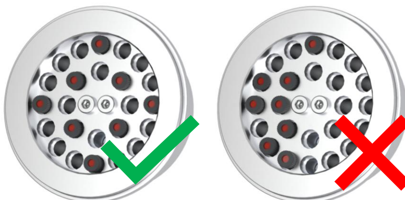
Fig. 65: Permissible arrangement of the glass vials in the adapter
