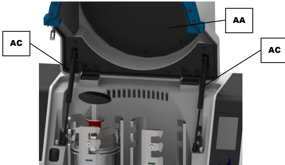
Fig. 69: Maintenance of the damper in the housing lid
