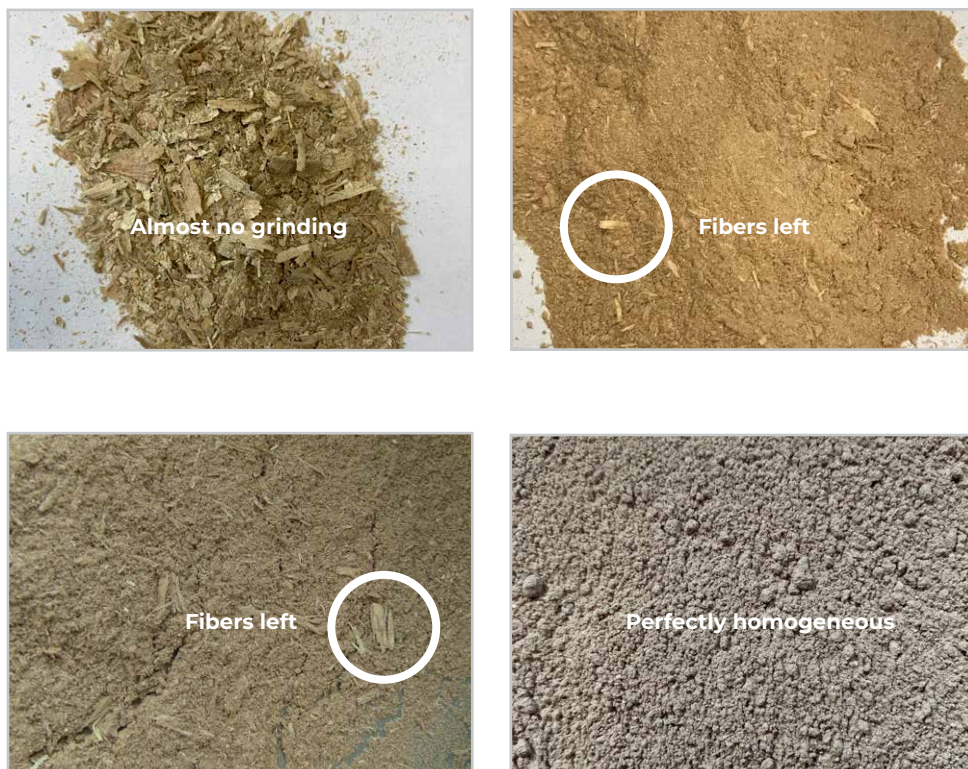
Fig. 9: Grinding results of dried plant samples in the different jar geometries in the PM 100 and PM 300. Images on the left: sample milled in old jar design (PM 100) Images on the right: sample milled in new flat jar design (PM 300) with better results
