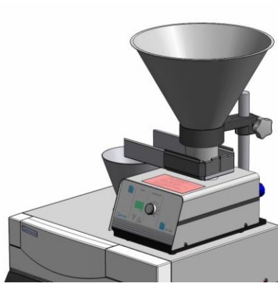
Fig 12: Assembly of the vibratory feeder
