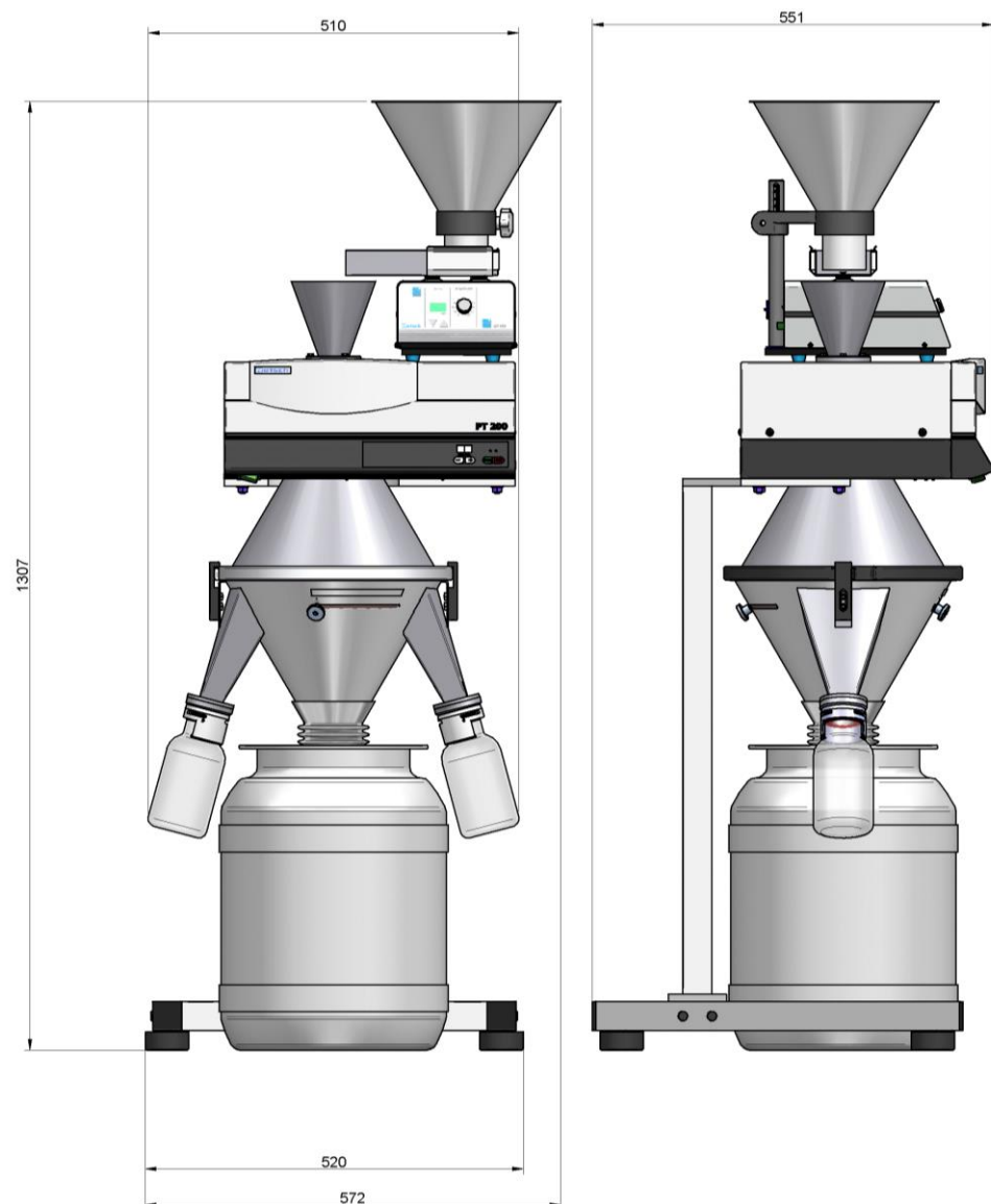
Fig. 2: Dimensions PT200 incl. sample divider
