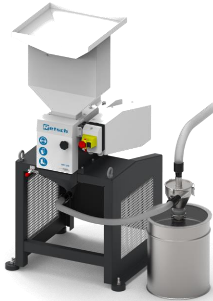
Fig. 22: HM 200 with connected cyclone, drum and vacuum cleaner
