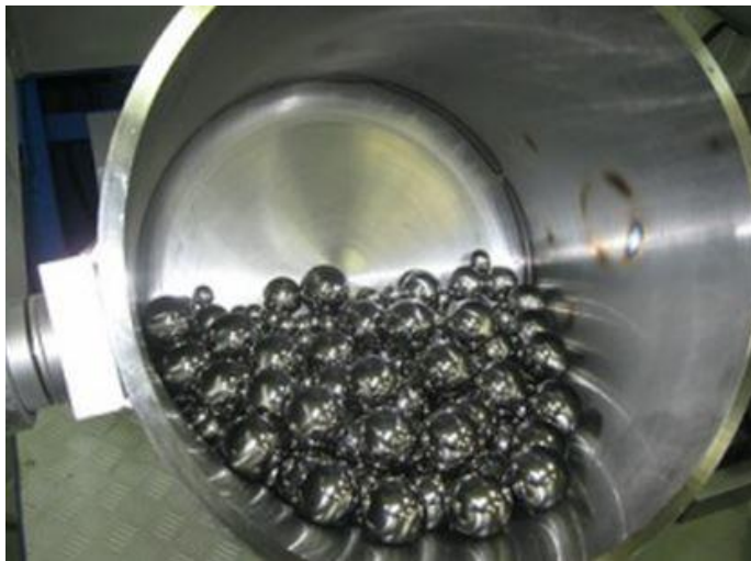
Fig. 17: Positioning the grinding balls
