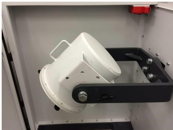
Fig. 24: Grinding drum in the emptying position
