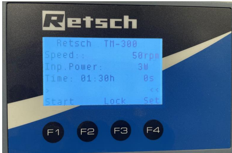
Fig. 28: Start menu – Housing door not locked
