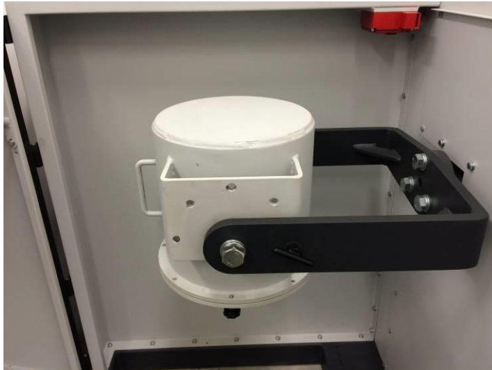
Fig. 25: Grinding drum in the complete emptying position
