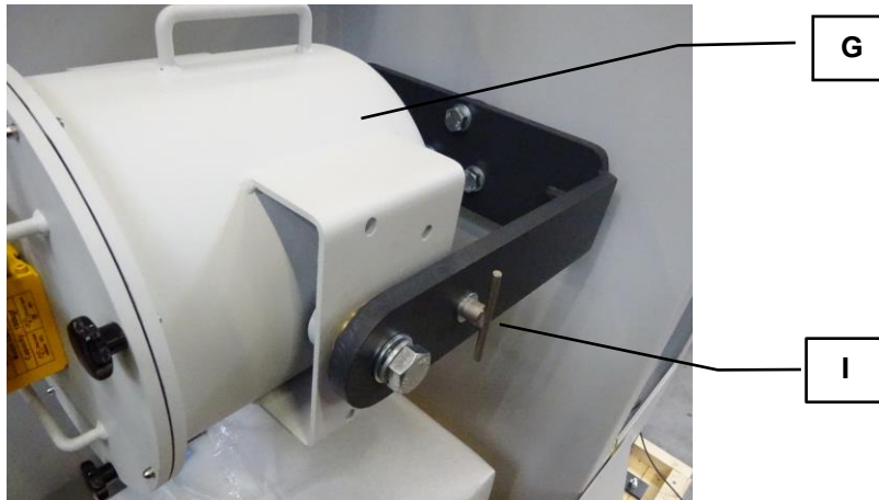
Fig. 10: Fixing the grinding drum with the locking screw
