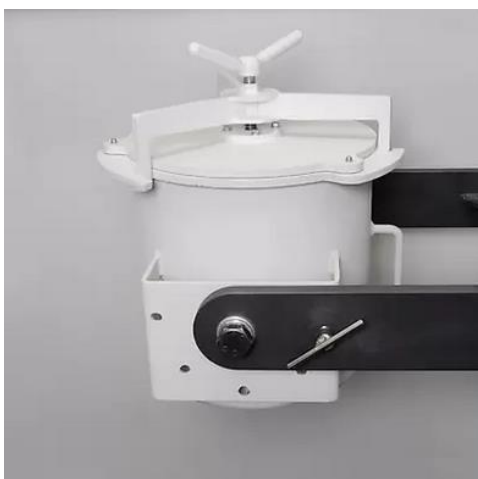
Fig. 19: Grinding drum with closed lid
