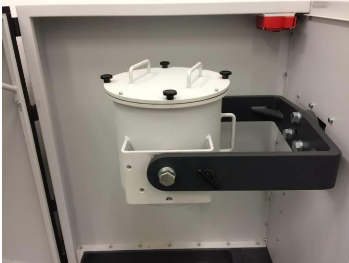
Fig. 16: Grinding drum (21.7 litres) in the filling position
