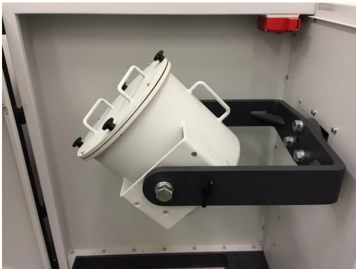
Fig. 22: Grinding drum in the mixing position
