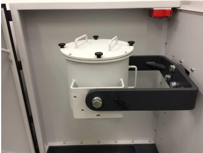
Fig. 21: Grinding drum in the filling position
