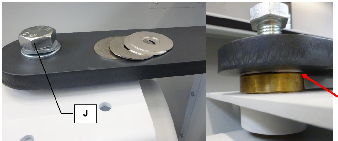
Fig. 11: Compensate the gap between the grinding drum and the grinding drum support
