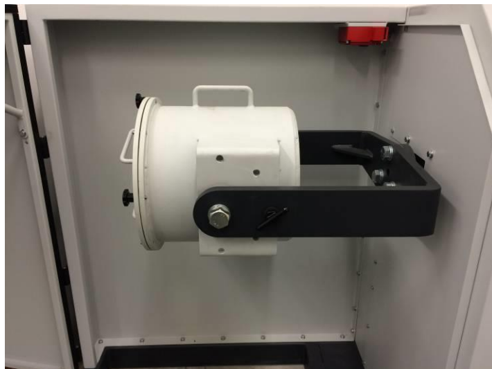
Fig. 23: Grinding drum in the grinding position
