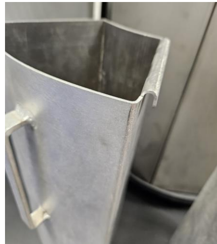
Fig. 16: Connection of partial segments by means of hooking them into each other
