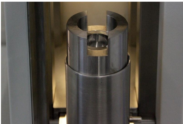
Fig. 23: Pressing tool for steel rings
