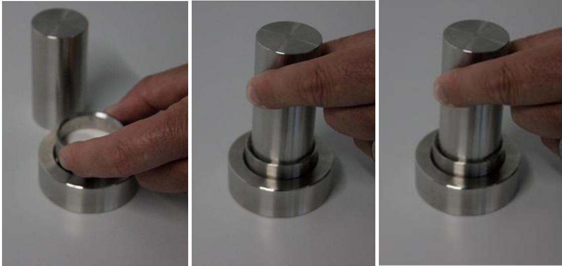
Fig. 26: Remove sample out of the steel ring.
