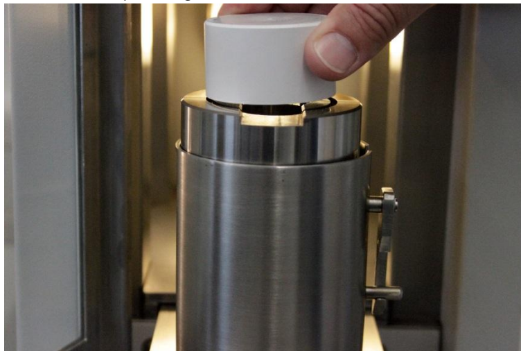
Fig. 18: Put on the pressing-out aid
