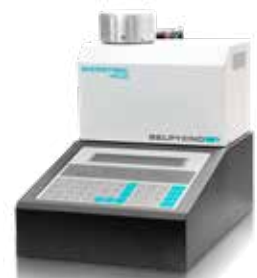
GASPYKNOMETER BELPYCNO L
