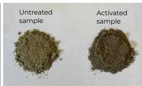
Figure 1: Sample process in a planetary ball mill PM 100. The parameters used are listed; The jar filling situation can be seen on the left; and an untreated and activated sample is shown. (source: Department of Architecture & Civil Engineering, Centre for Climate Adaptation & Environment Research, University of Bath).
