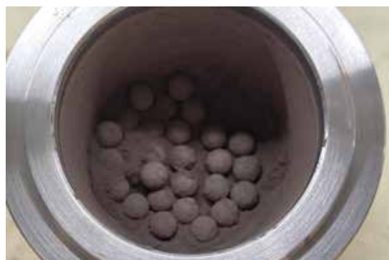
Figure 1: Sample process in a planetary ball mill PM 100. The parameters used are listed; The jar filling situation can be seen on the left; and an untreated and activated sample is shown. (source: Department of Architecture & Civil Engineering, Centre for Climate Adaptation & Environment Research, University of Bath).
