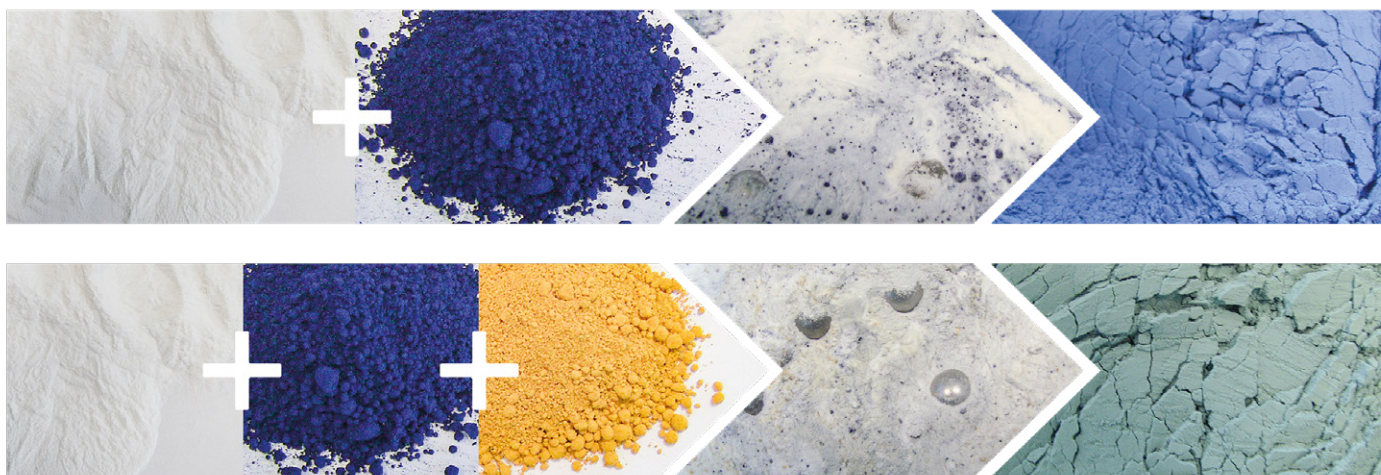
Top: Starch and blue Pigment after 5 minutes of milling in the PM 400 Bottom: Starch, blue & yellow pigment after 5 minutes of milling in the PM 400
