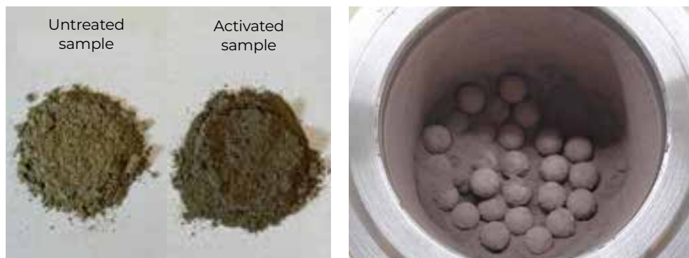
Figure 2: Sample processed in the Planetary Ball Mill PM 100 Speed: 500 rpm, Grinding Jar: 500 ml, Stainless Steel Grinding Balls: 12 × 20 mm, Stainless Steel, Ball-Powder-Ratio: 25:1
