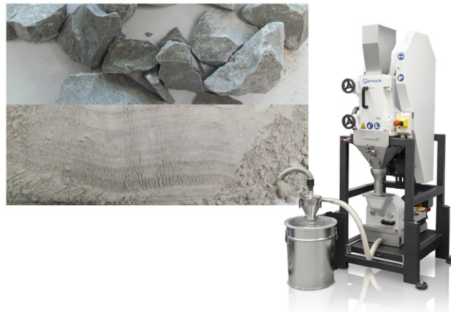
Figure 3: Combination unit consisting of Jaw Crusher BB 250 and Disk Mill DM 200 with cyclone, shown here with an application example for limestone.
