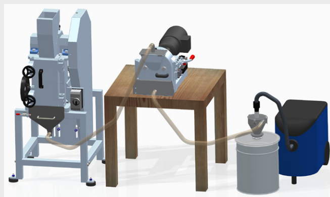
Machine 1 - Outlet - Hose/Steel connection tubing - Inlet - Machine 2 - Outlet - Hose/Steel connection tubing - Cyclone - Vacuum cleaner
