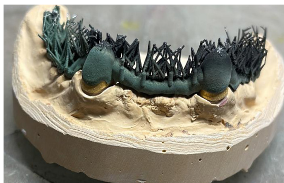
Fig. 4: Oxide layer on a model part before sandblasting
