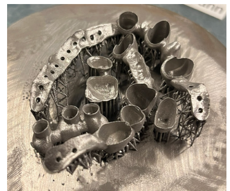
Fig. 3: Model view after 3D manufacturing
