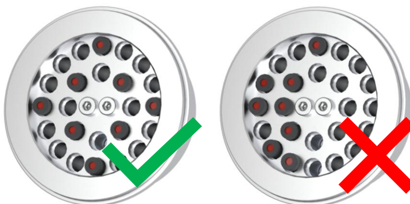
Fig. 28: Permissible arrangement of the glass vials in the adapter
